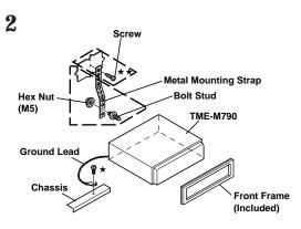
Reinforce the monitor with the metal mounting strap (not supplied). Secure the ground lead of the unit to a clean metal spot using a screw  $(\star)$  already attached to the vehicle's chassis.
